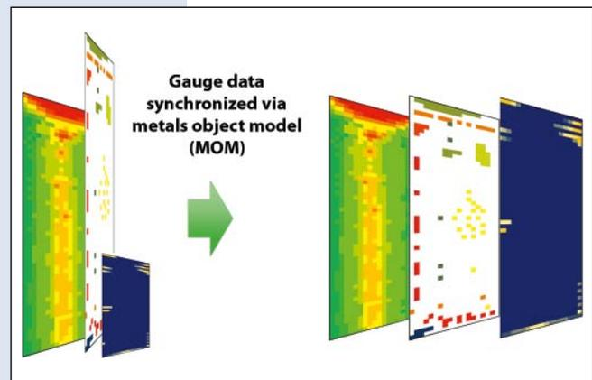
the rule application to certain coil sections (e.g. top side or head section) as well as to certain grades, customers or process lines. The individual results are tied together to a complete coil result with selectable criteria (e.g. worst rule result determines coil result). Rules can also trigger individual actions, e.g. sending a telegram (alarm notification). This mechanism also allows the “misuse” of rules to monitor process conditions (conditional monitoring system – CMS).
